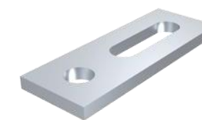
ZJ-AP-82x30A Material : AL6005-T5 Length : 82mm Surface Finish : Silver/Black anodized
